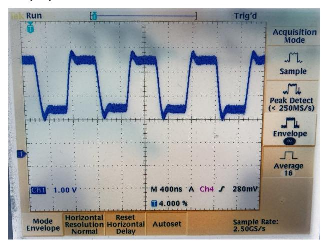
From the above scope trace, at 400ns/division, the minor grid dots correspond to 80ns each. The vertical transitions of the summed pulse train are less than half a grid dot, or < 40ns jitter. But, we can do better by zooming in to a single output pulse.
