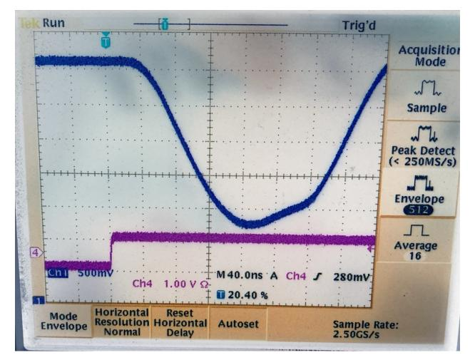
At 40 ns/div, the minor ticks correspond to 8 ns. For both the falling and rising edges, the envelope of the trace can be seen to be less than one minor tick. A reasonable upper bound on the jitter is about < 5ns jitter.
