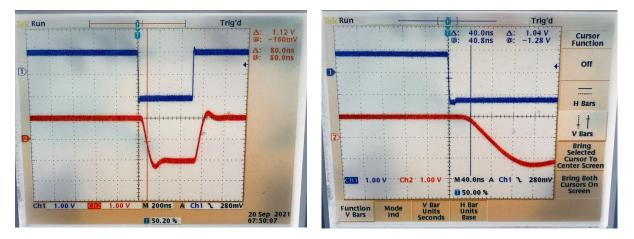
From the first trace, the propagation delay from input to the 50% output point is seen as 80 ns; while the second trace shows the delay from the input to the beginning of output transition of about 40 ns. This initial delay of 40 ns corresponds to the small-signal propagation delay of the SIM980; the additional 40 ns to reach the 50% point is due to the 40 V/ $\mu$ s input slew rate limit of the SIM980.
